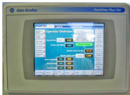
Allen Bradley PanelView Plus Touchscreen
